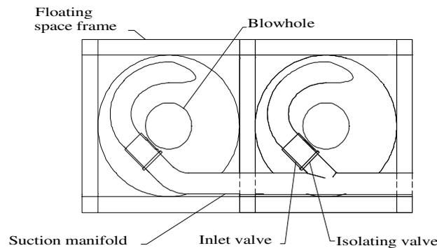
**Oscillating Water Column Detail**
