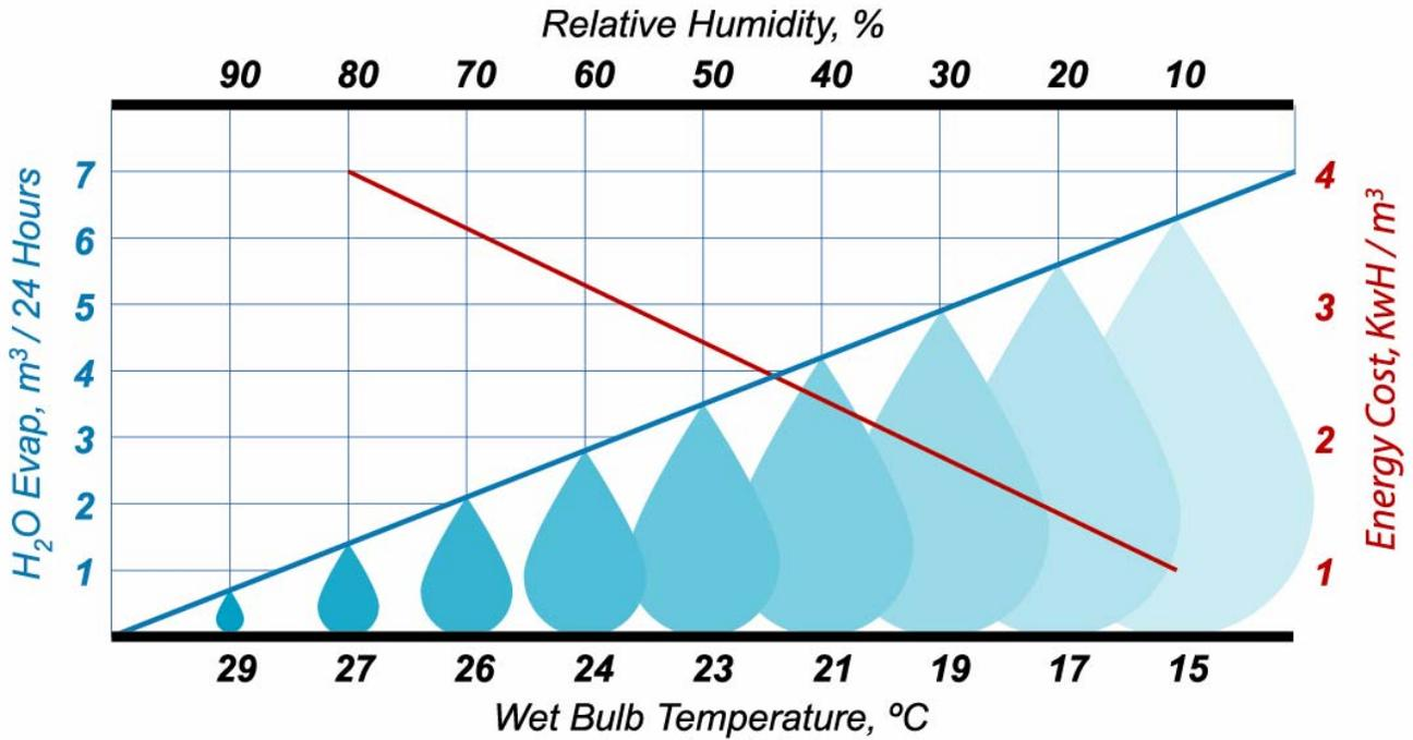
The chart illustrates the cooling effect and potential for evaporation for air at a constant temperature of 30°C with reducing humidity. The values are based on a nominal 1000 m<sup>2</sup> Seawater Greenhouse.
