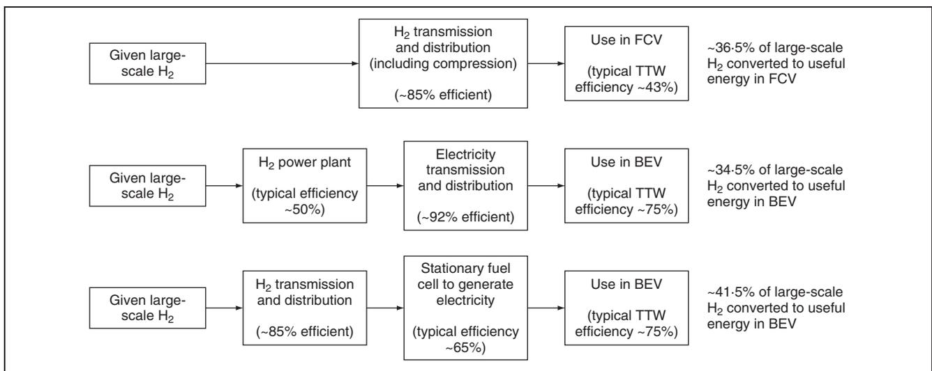
Fig. 2. Some examples of large-scale hydrogen use for BEVs and FCVs
