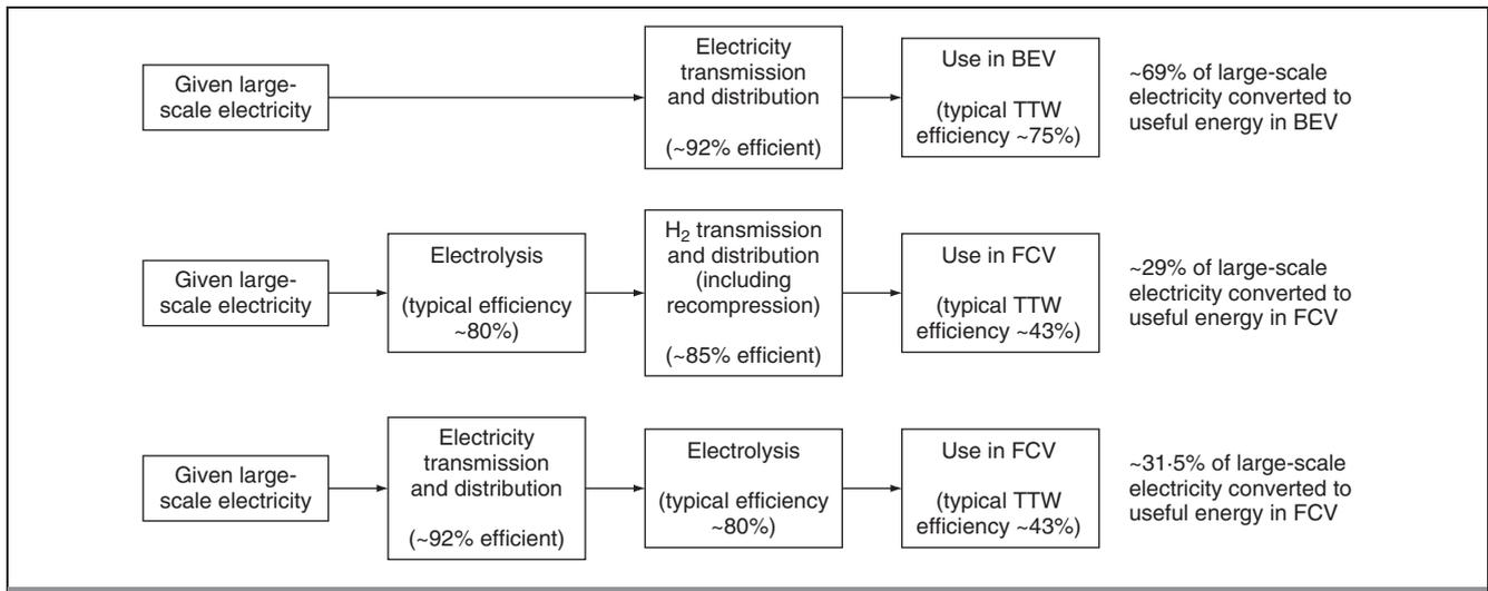
Fig. 1. Some examples of large-scale electricity use for BEVs and FCVs
