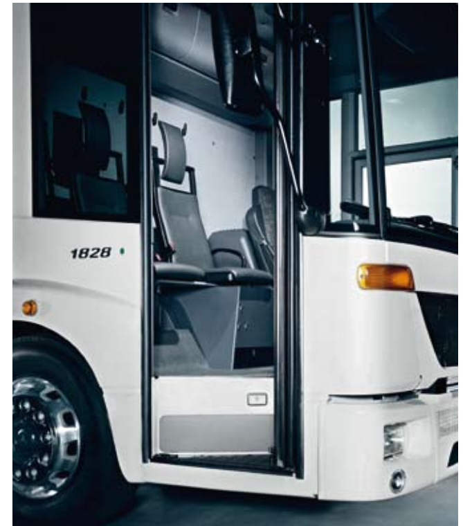
The Econic standard cab with full standing height and a level floor throughout makes for easy boarding and alighting. It offers space for up to three co-drivers in addition to the driver
