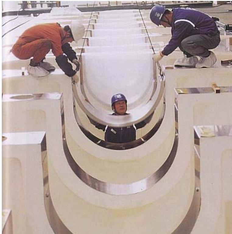
The crank sitting in the block (also known as a "gondola-style" bedplate). This is a 10 cylinder version. Note the steps by each crank throw that lead down into the crankcase:
