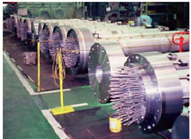
The "spikes" on the piston rods are hollow tubes that go into the holes you can see on the bottom of the pistons (left picture) and inject oil into the inside of the piston which keeps the top of the piston from overheating. Some high-performance auto engines have a similar feature where an oil squirter nozzle squirts oil onto the bottom of the piston.
